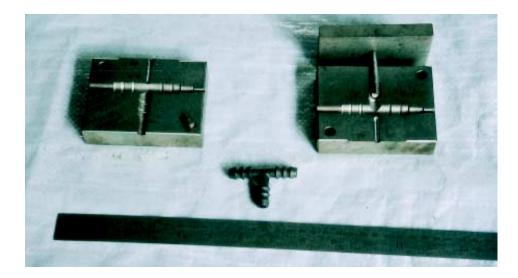
3. Double-Cavity Mould of 16mm End Cap:
