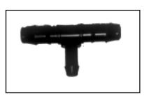
Tee Connector: Tee Connectors of various sizes are required in AMIT system to connect a branch to the Main pipe, Main pipe to Sub-main pipes, Lateral Pipes to Submain pipes etc. The Tee Connectors can be Equal Tee or Reducing type Tee viz. 12mm x 12mm, 16mm x 12mm, 16mm x 16mm, 25mm x 12mm, 32mm x 12 mm etc.
