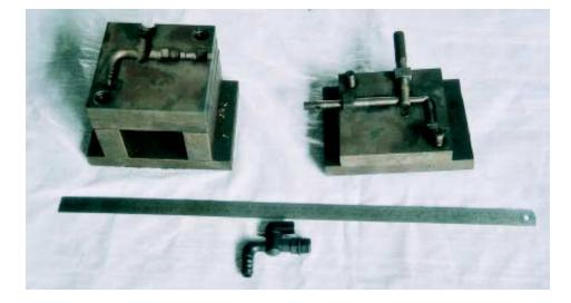
2. Single cavity mould of 16mm Equal Tee:
