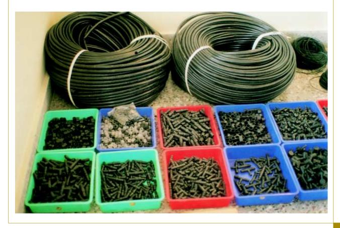
2. Required length of pipe being coiled after punching holes and fixing micro-tubes:
