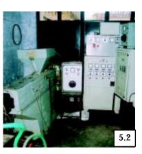
**4. Control Panels:** Control panels are required to maintain the temperature, speed of the motors for haul off, screw barrel, and voltage etc. As shown in picture 5.2.
