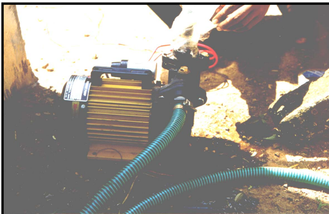
One 0,5 HP pump can operate two sprinklers (see page 7) at a time and replace a 5 hp pump
